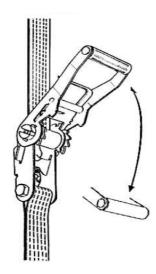
2. Pump handle to tension, ensure that there are a minimum of 1 ½ turns of webbing on the ratchet spindle
